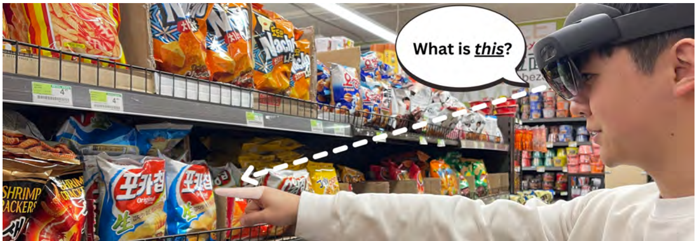
Figure 1: An example interaction with GazePointAR. The user’s query “What is this ?” is automatically resolved by using real-time gaze tracking, pointing gesture recognition, and computer vision to replace “ this ” with “ packaged item with text that says orion pocachip original ,” which is then sent to a large language model for processing and the response read by a text-to-speech engine.
